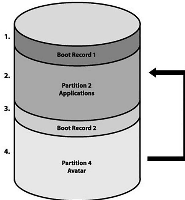
This diagram demonstrates how a multi-boot workstation can use “hidden partitions” to operate a backup operating system with Avatar. The Avatar system can then be used to maintain the baseline configuration of the primary partition. The advantage of this configuration is that even if the primary operating system is completely non-functional it can be returned to baseline configuration.
