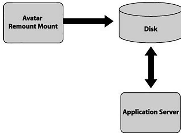
This example is the inverse of example 2. In this example the application disk is attached to the Avatar server and shared out to the Application Server.
