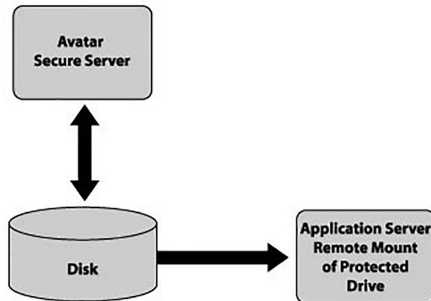
In this example, a secure server has been setup to run Avatar. The application server disk drives are shared using a secure protocol to the Avatar server. Avatar controls the baseline configuration of the application server remotely over the network. If the Application server disk share “disappears” then standard off the shelf software will sound an alarm.
